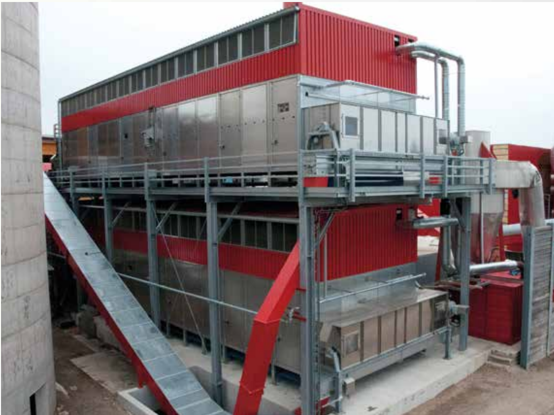
Project: German Pellets Germany Type: 2x BT 1/6200-22.5 Year: 2010 Product: Sawdust Dryer output capacity: 2x 6.5 t/h from 50% - 10% MC
