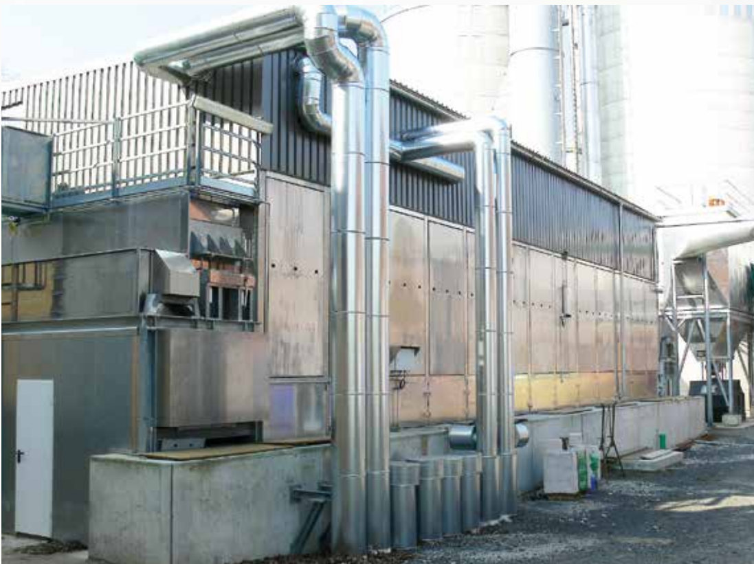
Project: EVO Energie- versorgung, Germany Type: BT 1/6200-19.5 Year: 2010 Product: Sawdust Dryer output capacity: 6.0 t/h from 50% - 9% MC
